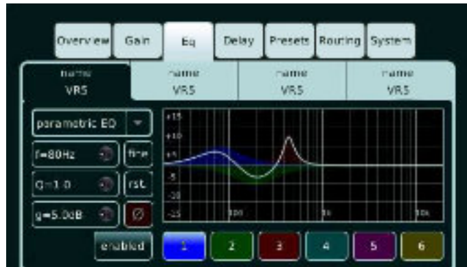
Fig 7. EQ Frequency adjustment per channel
