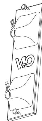
RC-X3 rain-proof protection for the amplifier section
